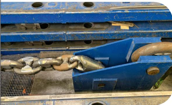
It is capable to withstand side loads during installation. It has a FEA proven design for inline and side loads.
